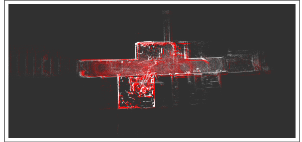
Fig. 8. Map created with 2 LiDAR frames matching
