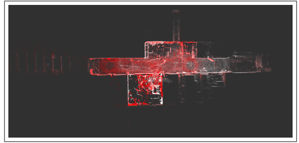
Fig. 7. Map created with 1 LiDAR frame matching
